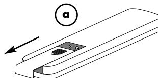
b) If necessary, remove used batteries and insert new ones correctly as shown by the diagram in the battery compartment.
