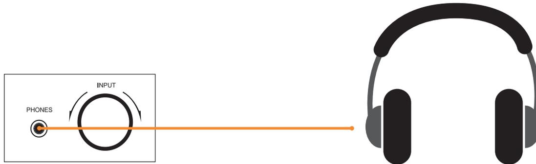
This will turn off the speakers. All headphones with impedance between 32 ohms and 600 ohms can be used. Inadequate headphones with too low impedance can damage the amplifier or unexpectedly produce such high volume that your hearing can be damaged. As a precaution, be sure to reduce the volume on the knob or on the "VOLUME" buttons (5/20) before inserting them.
