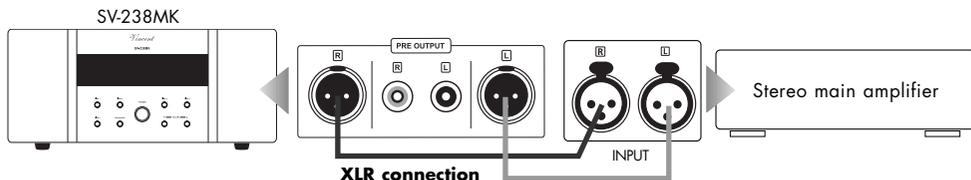
Both outputs reproduce the same stereo music signal of the currently selected source. Instead of the stereo main amplifier used here two mono main amplifiers can be utilized.
