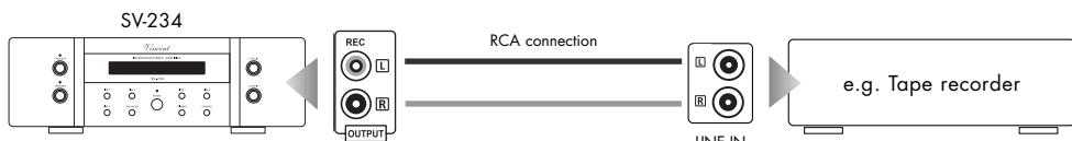
Connect this signal output to the signal input ("LINE IN", "TAPE IN" oder "REC IN") on the recording appliance using RCA cables. Please note that some recording equipment can have a slightly detrimental effect on the audio signal quality. Some recording devices have rather low input impedance, which can slightly alter the input signal voltage. For maximal music enjoyment we recommend that you connect to the "REC" terminal only for as long as the recording is actually being made.
